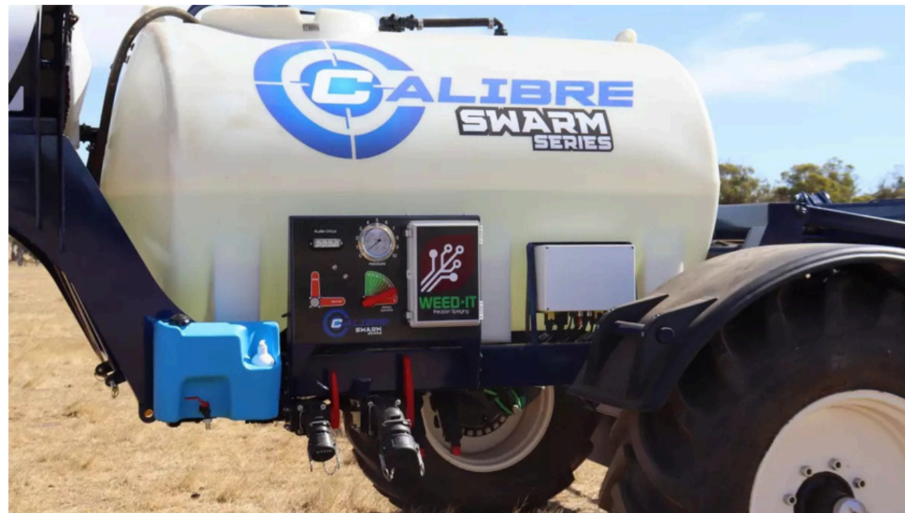
Joe is fitted with a 3000 litre main tank.
