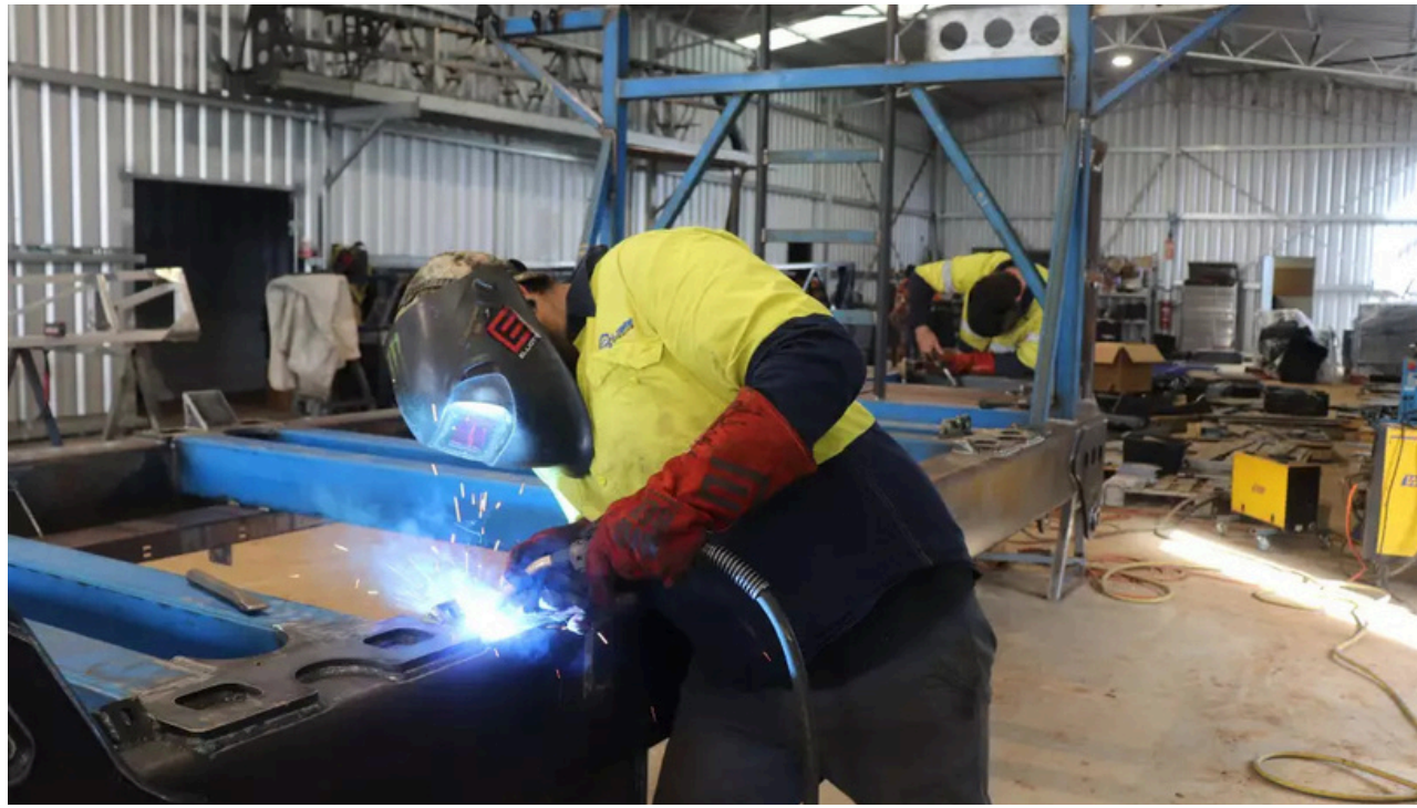
Welder Ashley Thurnwood working on a Calibre boom sprayer chassis at Eagle Eye Engineering.
