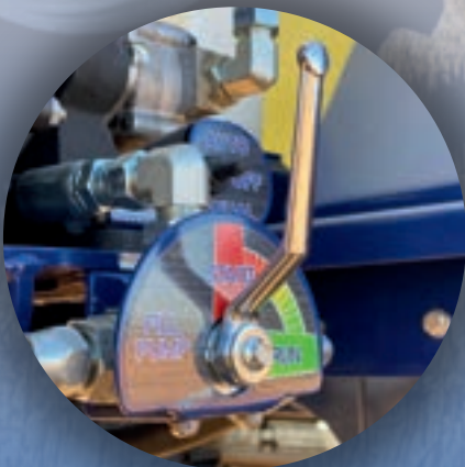
HYDRAULIC FILL CONTROL
